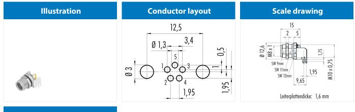
Contact arrangement (Plug-in side)
